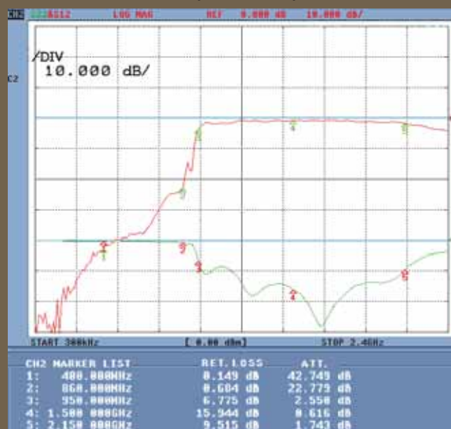
Tap SAT A/F response and return loss
