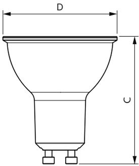
ESSLEDspot 6W 500lm GU10 827 120D ND RCA
