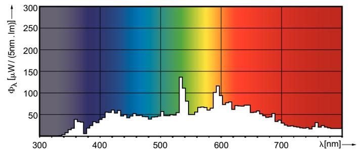
XDPB\_XDCDMSAT\_942-Spectral power distribution B/W
