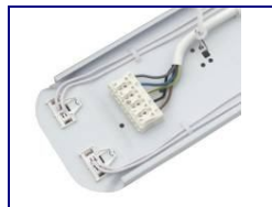
3LIN- Through wiring 5x1.5 mm 2 with two push-in terminal blocks (or 3LIN2,5- through wiring 5x2.5 mm 2 )
